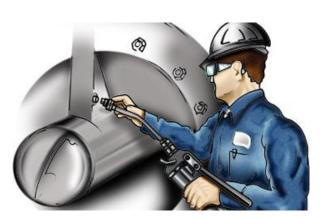
The separation of oil shall vary based on the storage time and temperature. The higher the storage temperature, the more are chances the oil will be released. Similarly, the lower the base <u>oil viscosity</u>, the more oil separation shall occur. Studies have also suggested that when the grease is in storage conditions, it is normal to have oil separation of up to 5 percent of the volume.
