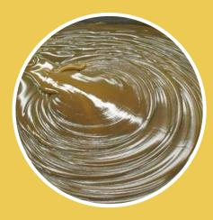
Grease bleeding is a kind of oil separation and an expression used to refer to grease that has released oil during storage. In steady conditions, oil bleeding is identified by the presence of small pools of oil, particularly when the grease surface is not flat or has a scoop removed out of it. In working conditions, it is distinguished by oil leaking from a lubricated component due to extreme pressure or heavily loaded condition.
