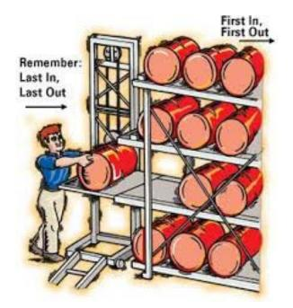
Bearing Lubricants cannot be stored in a dirty, dusty environment as they can be easily contaminated. Contaminated lubrication is not good for the business, whereas improved lubrication storage helps to achieve several benefits. So it is also important to store the bearing lubricants in a dry, cool and clean environment where containers can be easy to rotate and the use of the first-In, first-out technique would be easy.
