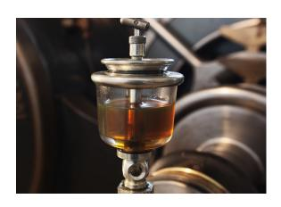
Condition monitoring will always help in avoiding sudden breakdown, Condition monitoring involves, control of contamination in the lubricant, filtration of oil, Analysis of lubricants used. Collection of sample getting it tested.
