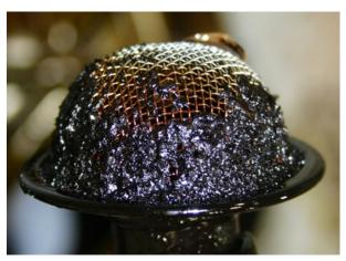
Heat can be generated from various sources such as metal to metal contact occurred due to improper lubrication, surrounding conditions etc. Separation of atoms and hydrocarbon occurs due to heat energy.
