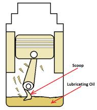
Splash oil feed system has a oil scoop directly resting on the shaft. The lower half of the ring is submerged in a oil reservoir located in the lower half of bearing housing. As the shaft rotates, the oil scoop turns carrying oil from reservoir up to the top of casing. The oil spreads across the shaft and bearings thus lubricating it and any excess runs back down into the reservoir.
