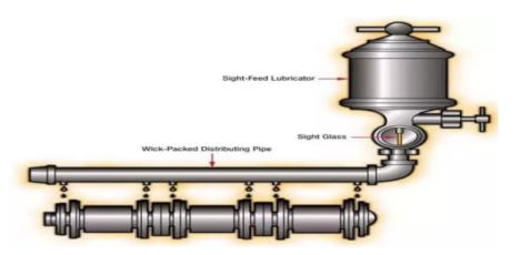
A drip feed reservoir connected to one bearing is called as single point system and when connected to several bearings is referred as multiple point systems. A drip oil feed system can also be pressurized to supply oil to bearing system under pressure. The reservoir is partially or completely transparent and can be refilled by hand.
